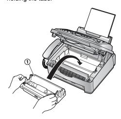
**10** Close the front cover (①) by pushing down on both sides, until locked.
